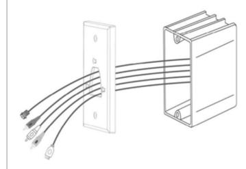
**2** Attach the cable pass-through panel to the electrical box with the two included mounting screws.
